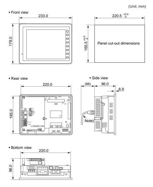
Note: Arrange SX bus expansion cable so that radius of bend in the cable is at least 50mm. Plug/unplug the SX bus expansion cable in the perpendicular direction.
